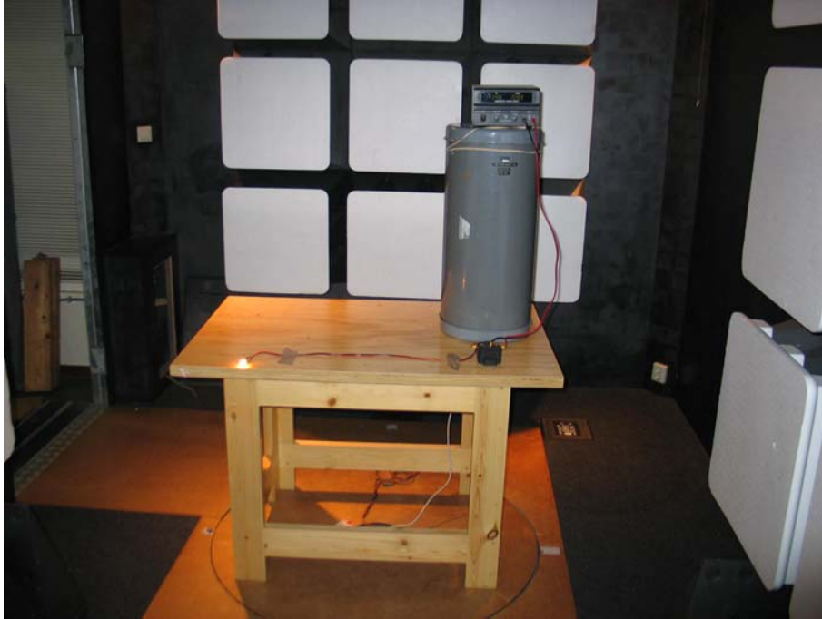
Photo 6. Basic set-up during radiated immunity tests) for EN 61000-6-2 requirements: EUT 1 (example set-up for all models)
