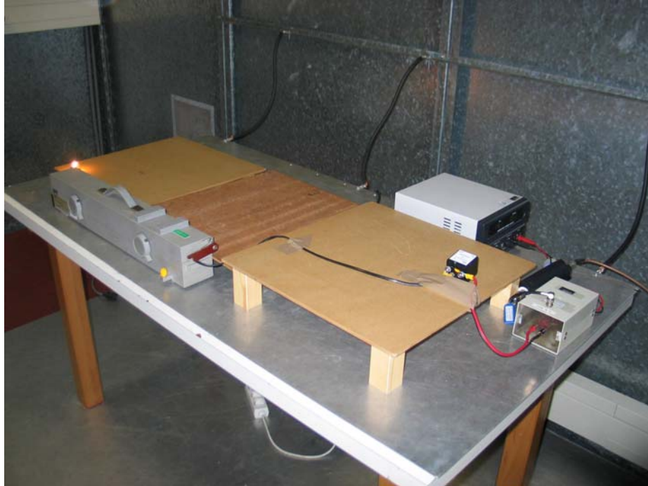
Photo 7. Basic set-up Conducted Immunity on DC input line of EUT1, EUT2 and EUT 3 (EUT2 as example).
