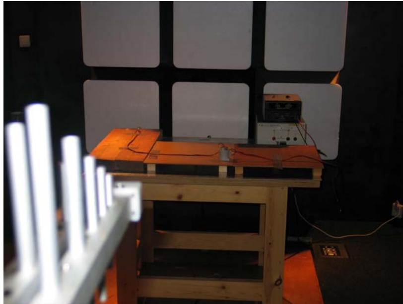
Photo 5. Basic set-up during radiated emission (and immunity tests) for automotive requirements: BS250 (example set-up for all models)
