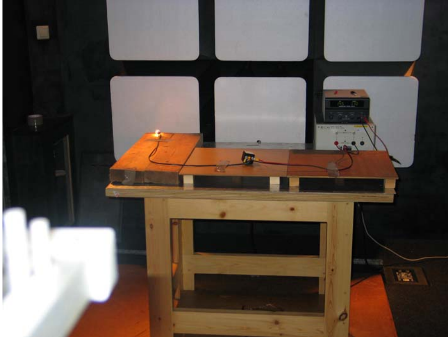
Photo 8. Basic set-up radiated Immunity of EUT1, EUT2, EUT 3 and EUT 4 (EUT2 as example).
